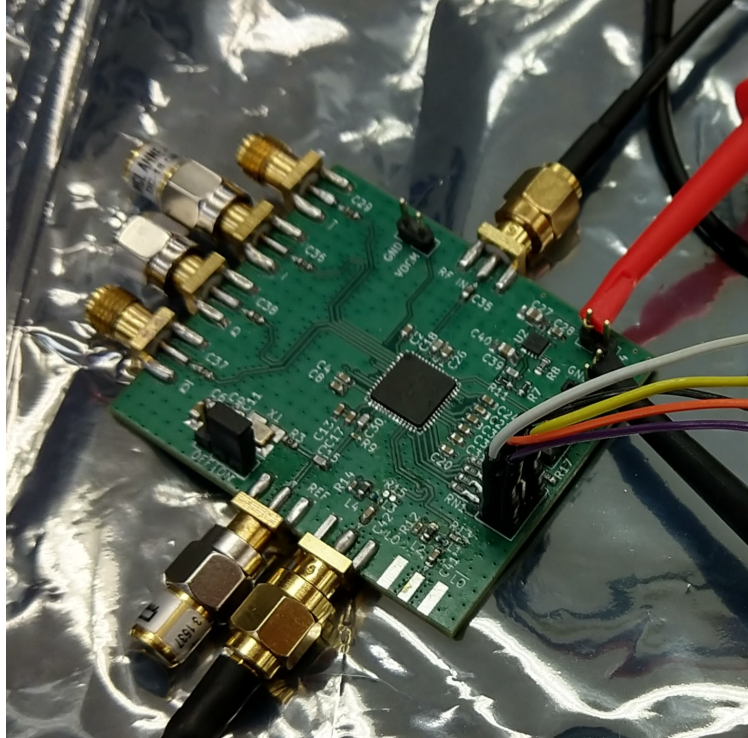
Figure 9: Receiver board and LO test connections
